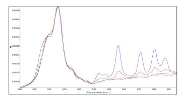
**Figure 3.** FT-Raman spectra for placebo (purple curve) and EVA/E2 extrudates containing 0.3% (green curve), 2.5% E2 (red curve), or 10% E2 (blue curve) between 680 and 470 cm<sup>-1</sup>.
